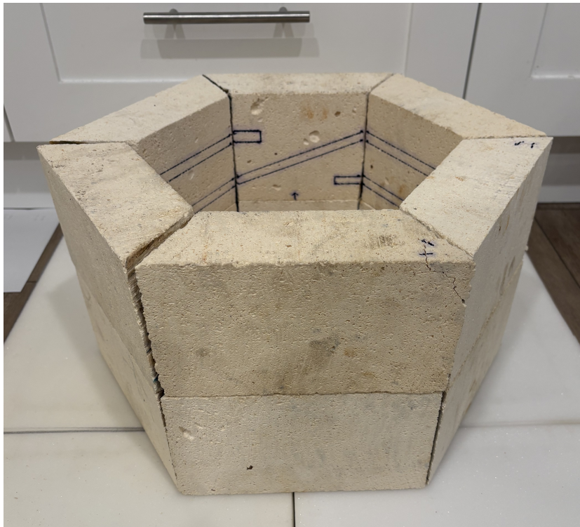
Figure 9.3: Dry-fit chamber assembly with element groove channel paths marked on the brick faces prior to cutting.
