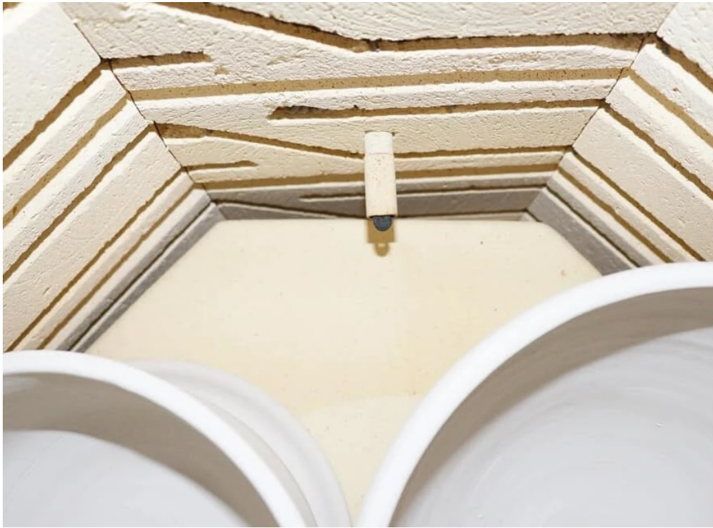
Figure 7.2: Example photo showing ideal thermocouple placement in a kiln firing chamber.
