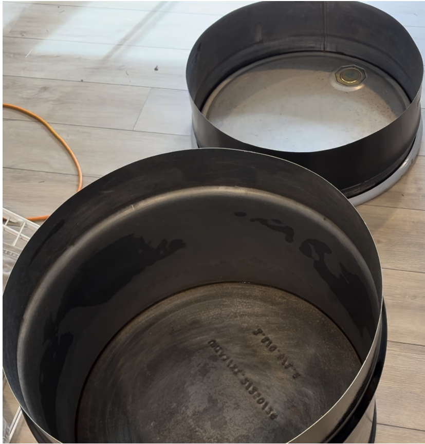
Figure 9.6: Barrel after cutting, showing the separated lid and chamber sections sized to match the insulation stack and chamber heights.
