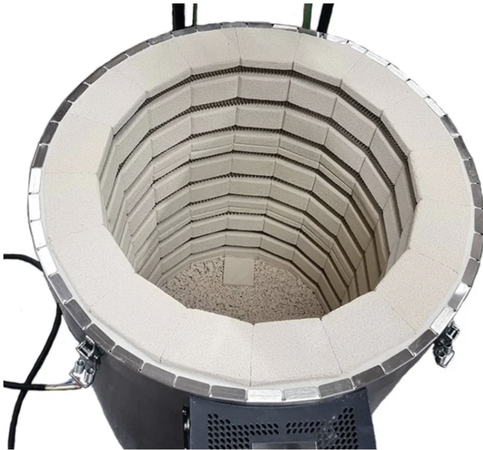
Figure 5.4: Example of bent metal tab lid support design of the chamber edge. The lid section edge will also use this strategy to retain the brick slab.
