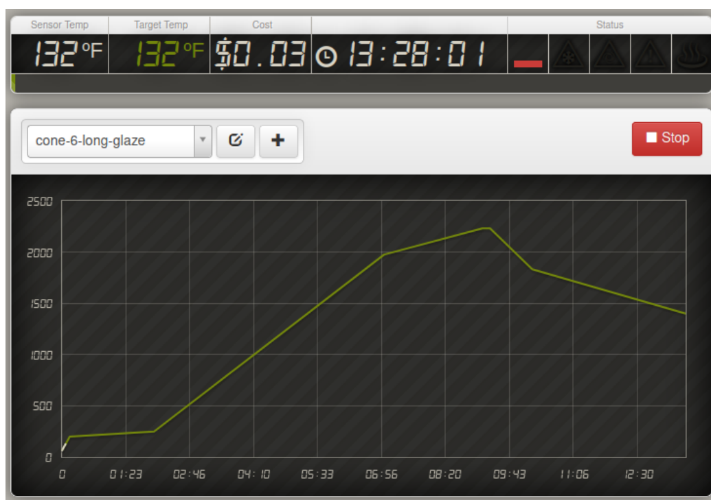
Figure 7.4: Example image of the Web UI of the kiln controller software, as accessed over the local network.
