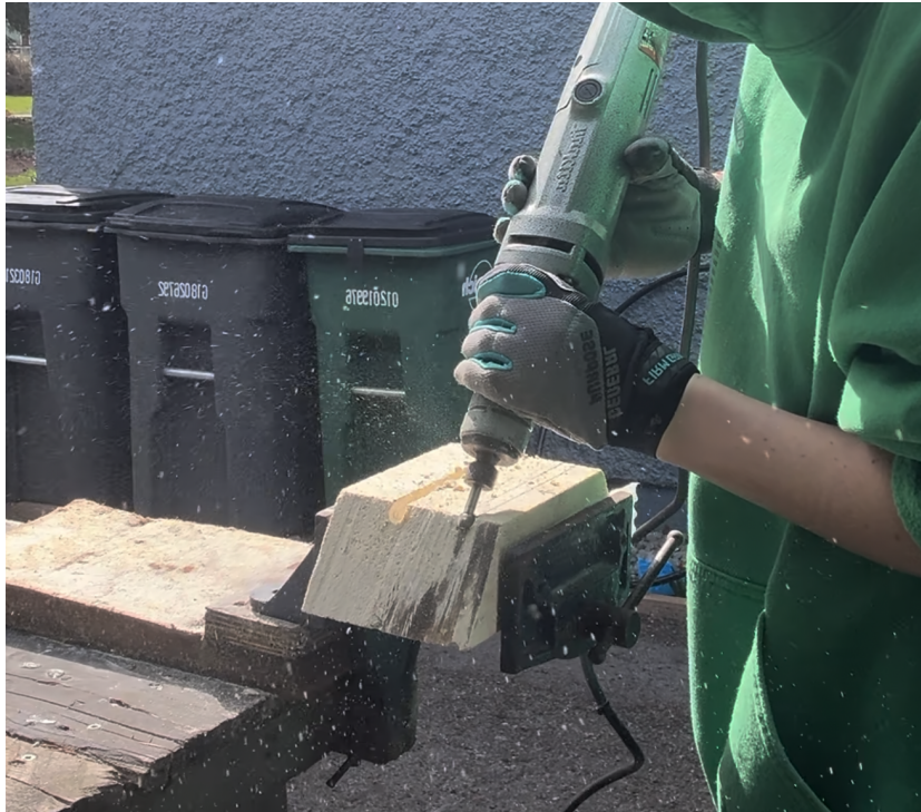
Figure 9.4: Die grinder with spherical bit used to cut the undercut element grooves into the IFB sidewall bricks.
