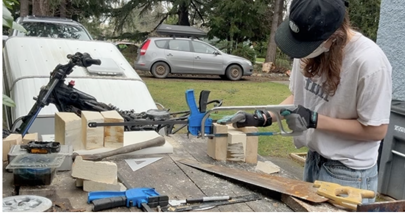
Figure 9.2: Hacksaw used with the bevel-cutting jig for IFB cuts; the large-tooth wood saw used for the majority of cuts is also visible.
