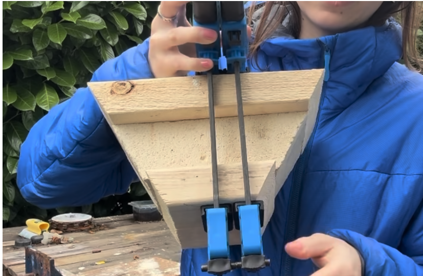
Figure 9.1: Bevel-cutting jig clamped around a cut IFB chamber brick during sidewall fabrication.
